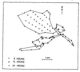
Figure 6. Notional particle tracking at points o before the storm then after 12 hours they would be located at  $\Delta$  and after 24 hours they would be at  $\alpha$
