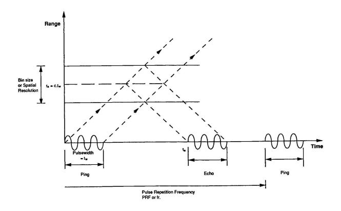
Figure 3. Time/Space diagram for a transmitted pulse
