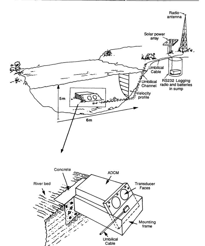
Figure 1. Typical Deployment of ADCM
