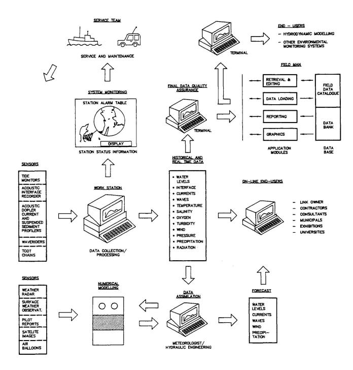
Fig. 2 Hydrographic Information System Setup.
