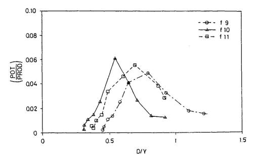
Fig. 3 Measured entrainment efficiency ratio in three experiments. The actual device is a barge without a propeller attached. Each experiment starts with high D/Y values. As the mixing takes place, the interface moves downward and the D/Y values become smaller.
