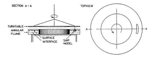
Fig. 2: Sketch of the experimental setup.
