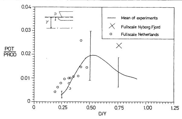
Fig. 4: Entrainment efficiency measurements POT/PROD as function of D/Y for a propeller-powered ship in force balance, i.e. |Fprop| = |Fdrag|. The line indicates the mean value and the error bars the standard deviation of the laboratory experiments. Results from full scale measurements are plotted for comparison.
