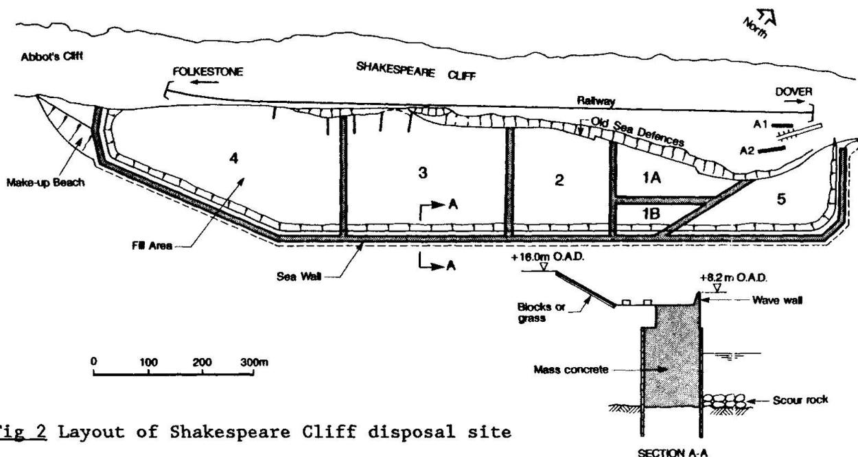
Fig 2 Layout of Shakespeare Cliff disposal site
