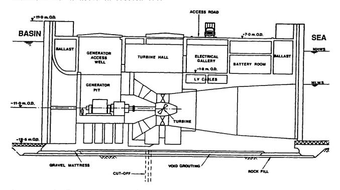
Figure 3 - Turbine-generator caisson
