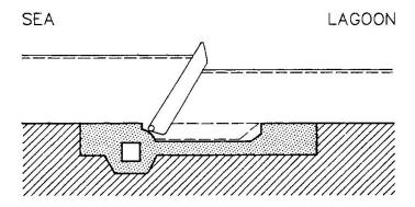
Fig. 2. Sketch of the proposed floating gates.
