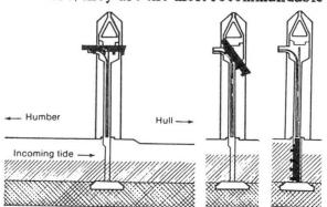
Fig. 3a: HULL lifting storm surge barrier.
