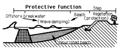
Fig. 2: Conceptual Diagram of the Zonal Protective Method.
