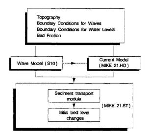
Fig. 3. Overview of the parts of the MIKE model complex used for calculation of initial bed level changes.
