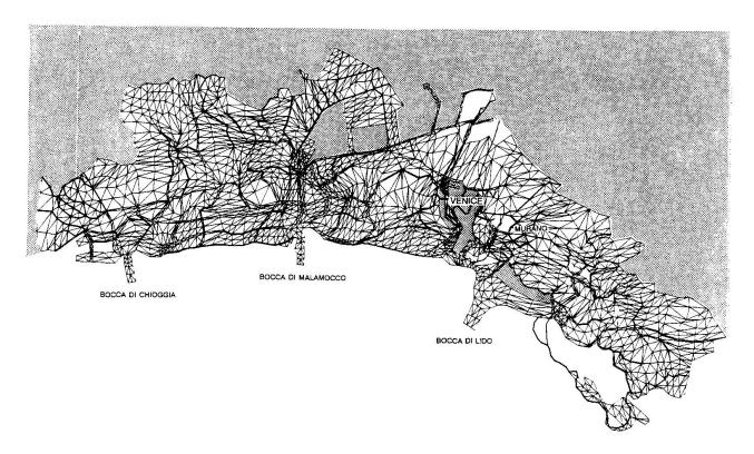
Fig. 4 The mesh of the two-dimensional finite element mathematical model.
