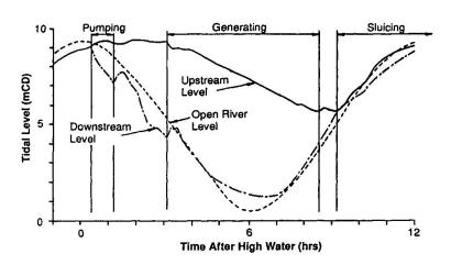
Figure 5 - Operating Water Levels - Spring Tide
