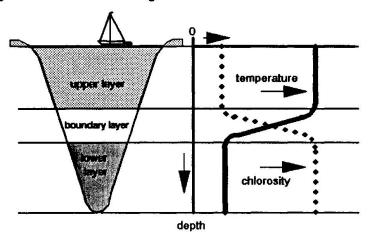
fig.2 Scheme of salt and temperature stratification
