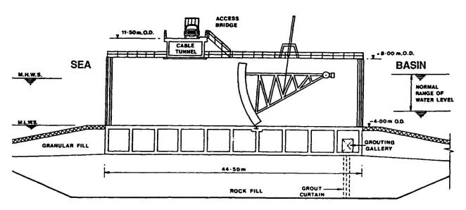
Figure 4 - Sluice caisson
