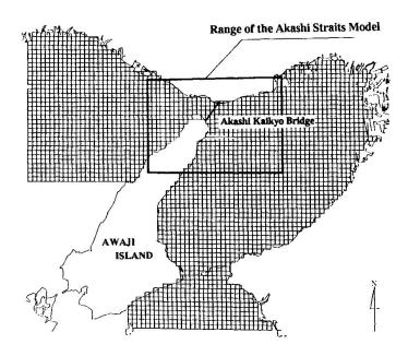
Figure 3 Mesh diagram for the Osaka Bay Model
