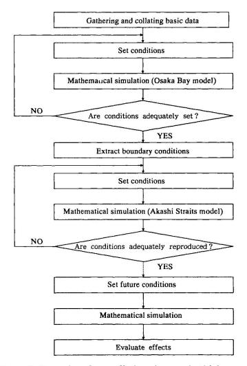
Figure 2 Procedure for predicting changes in tidal current
