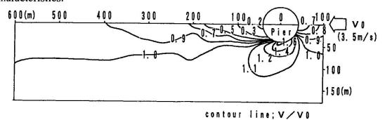
Figure 7 Flow around a circular pier
