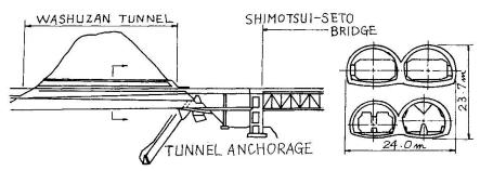
Fig.2 Side view and cross section of Washuzan Tunnel
