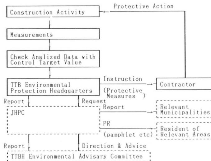
Fig.1 Environmental surveillance and protection procedure during construction
