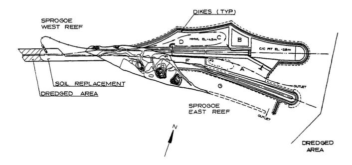
Fig. 2 Sedimentation basins at Sprogoe.
