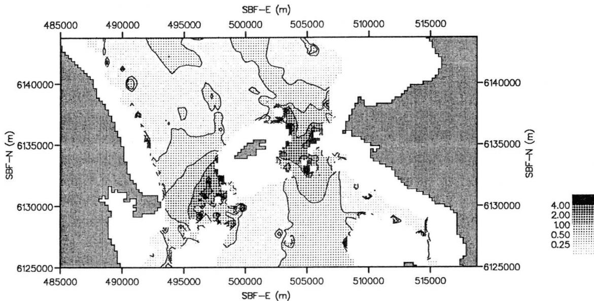
Fig. 13 Contour plot of Froude number (07/09/89, 02:00). In blank areas one layer flow is present due to shallow water depth.
