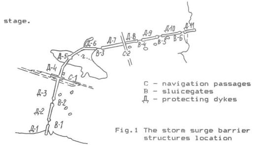
Out of the total length of the barrier only the fraction 0.9 km long remains undeveloped. It is there that the main navigation fairway goes. So far the construction of the main navigation passage has not been completed either. All the six sluicegates provided for by the desin are in operation, the sluices are fitted with 64 big gates and spans 24 meters long(Fig.2).
