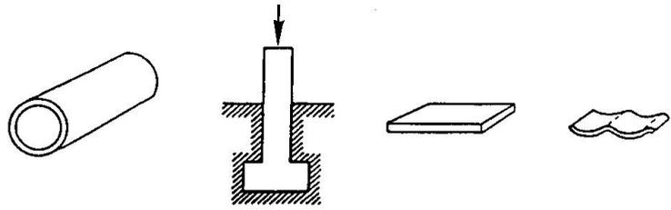
**Fig.4** Examples of the use of unreinforced concrete
