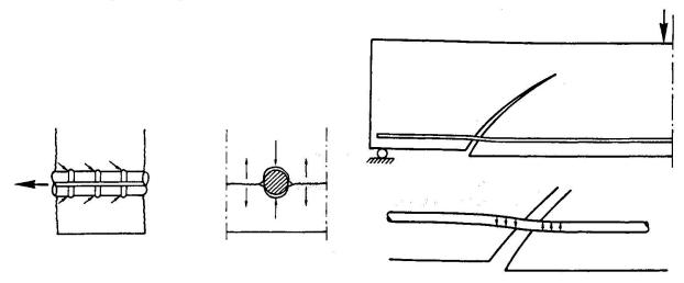
Fig.1 Splitting forces from reinforcement and possible tensile cracks
