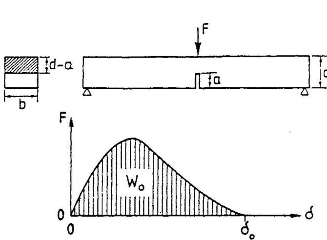
Fig. 7 A stable bending test on a notched beam with registration of the load-deflection relation for the determination of  $G_F$  according to RILEM [7]
