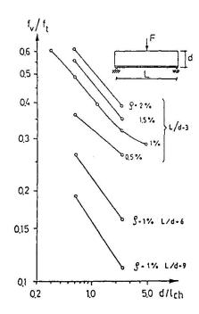
Fig.11 Theoretical ratio between a formal flexural strength and the tensile strength for two different types of failure of an unreinforced concrete pipe
