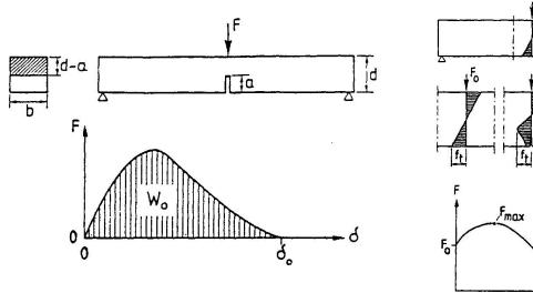
Fig.7 A stable bending test on a notched beam with registration of the load-deflection relation for the determination of G<sub>F</sub> according to RILEM [7]
