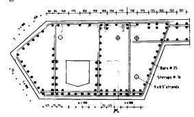
Fig. 7: Reinforcement in Edge Beam
