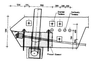
Fig. 11: Edge beam near cable anchorage
