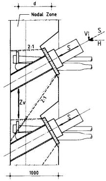
Fig. 4: Truss Action at Towerhead in elevation
