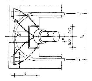
Fig. 3: Truss Action at Towerhead in plan
