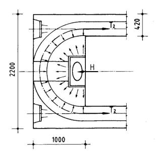
Fig. 5: Arch Action at Towerhead
