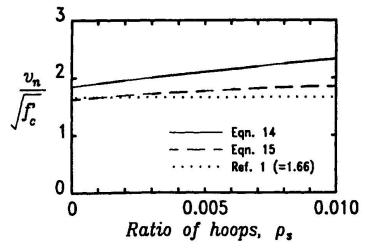
Fig. 3 Shear resistance after hoop yield
