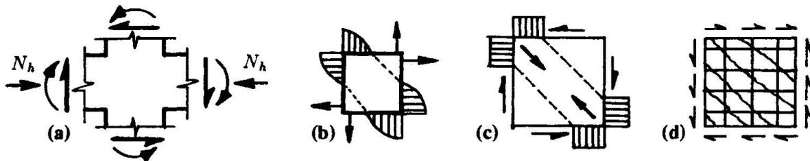
Fig. 1 Shear mechanisms adopted by design codes
