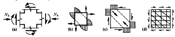
Fig. 1 Shear mechanisms adopted by design codes
