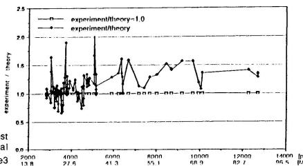
Fig. 2 Comparison of test results with theoretical approaches for predicting f<sub>ce3</sub>
