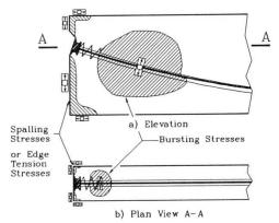
Figure 2: Tensile Stresses in the Anchorage Zone
