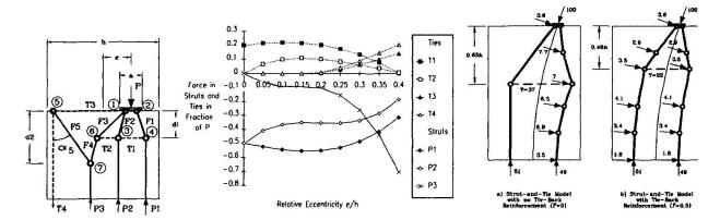
Figure 6: Strut-and-Tie Figure 7: Forces in the Struts and Ties as a Figure 8: Strut-and-Tie Model of an Model of an Eccentric Function of the Eccentricity
