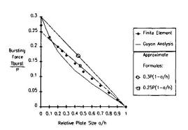
Figure 5: Bursting Force for Concentric **Tendons**
