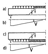
The form of the sections in both, B and D regions gives a direct interpretation of the required extension of the flexural reinforcement in presence of shear and of the staggering rules as well.
