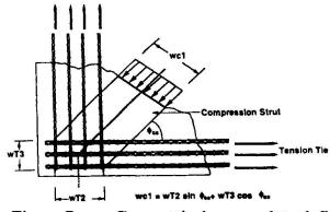
Figure 7 Geometrical approach to define the strut width for CTT-node
