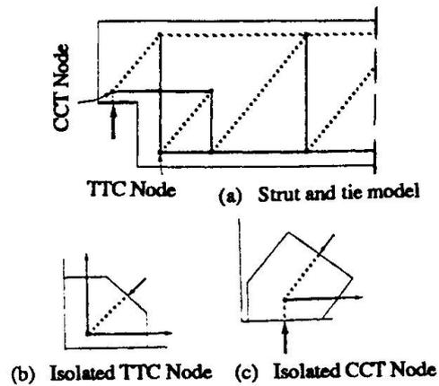
Figure 1 Strut and tie model of the prototype dapped beams.
