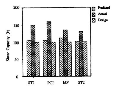
Figure 3 Comparison of specimen shear capacities.
