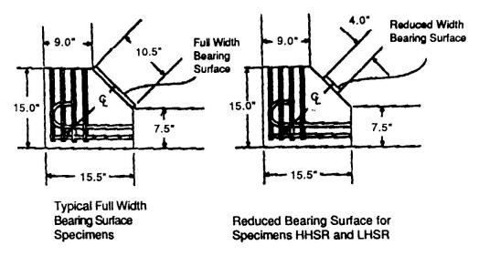
Figure 8 Typical CTT-nodes tested (from Ref. [4]).
