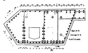
Fig. 7: Reinforcement in Edge Beam
