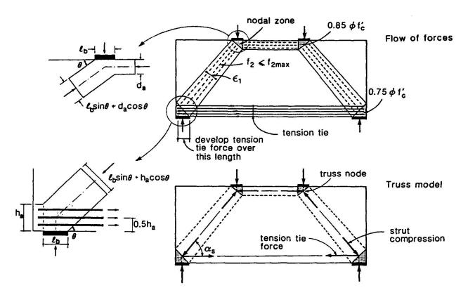
Figure 1: Strut and tie modeling of a deep beam.
