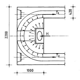
Fig. 5: Arch Action at Towerhead
