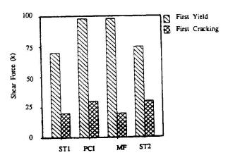
Figure 4 Comparison of cracking and yield loads
