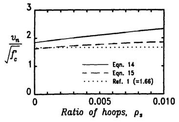
Fig. 3 Shear resistance after hoop yield
