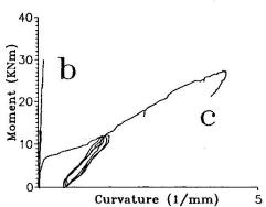
$\underline{\text{Fig.4}}$  - Evidence of the tension stiffening effect from the experimental results
