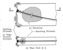
Figure 2: Tensile Stresses in the Anchorage Zone
