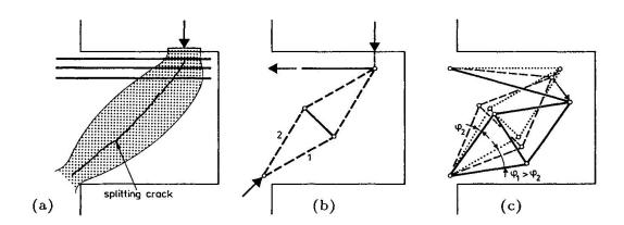
Fig. 5: Strut-and-tie model explaining diagonal splitting; (a) bottle compression field; (b) refined model; (c) deformation and rotation
