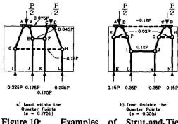
Figure 10: Examples of Strut-and-Tie Models with two Tendons
