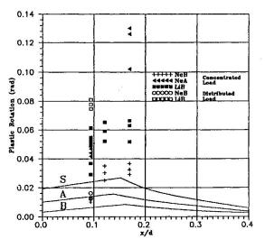
Fig.2 - Experimental plastic rotation
