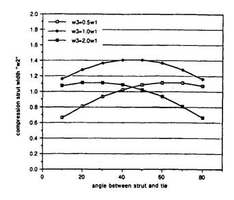
Fig. 3 Dependency of  $v_e$  for CTT-node
