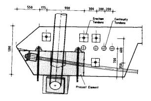
Fig. 11: Edge beam near cable anchorage
