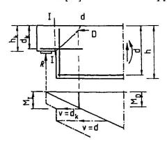
The flexural reinforcement at this corner must be dimensioned for the moment  $\mathbf{M}_{D}$  (under the point of application of the compressive inner force on the section d–d shown in Fig. 5a. Applying the horizontal shifts v and  $\mathbf{v}_{k}$  resp. due to the effect of the inclined shear crack, approximate the same moment is obtained under the conventional cross section I–I, which is to be dimensioned here actually.
