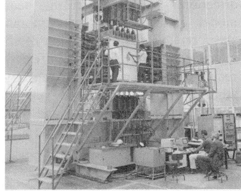
Fig. 5 University of Toronto Shell Element Tester
