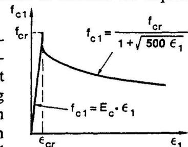
Fig. 3 Average Stress-Strain Relationship for Concrete in Tension
