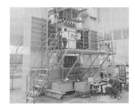
Fig. 5 University of Toronto Shell Element Tester
