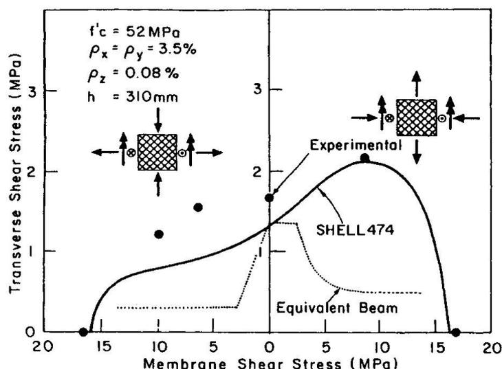
Fig. 6 Membrane Shear - Transverse Shear Interaction
