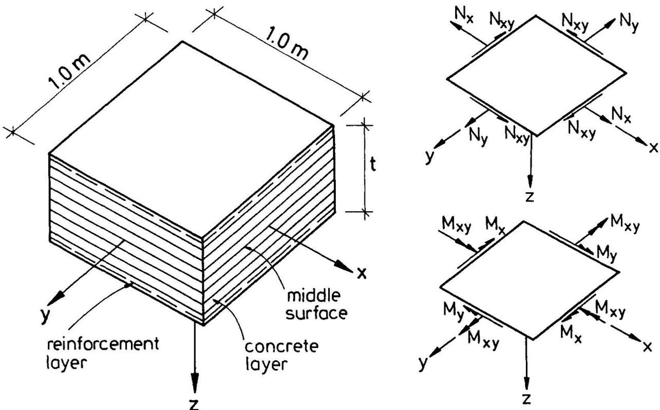
Fig. 1 Layered shell element (left), applied forces and moments (right)
