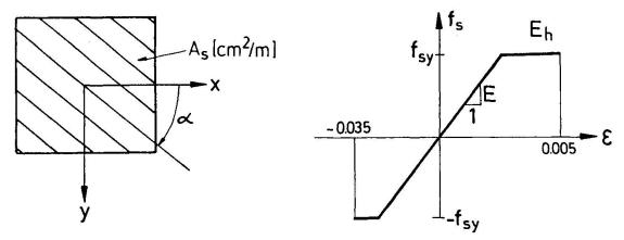
Fig. 3 Reinforcement layer and material model for the reinforcement
