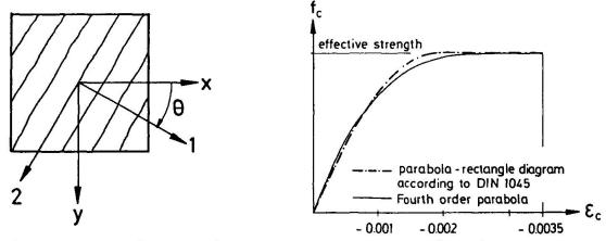
Fig. 2 Concrete layer with cracks in one direction (left) and uniaxial stress-stress strain diagram of concrete (right)
