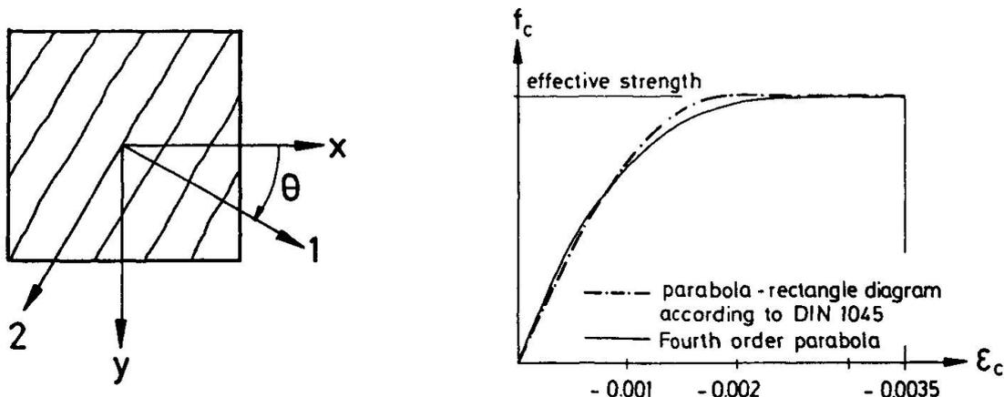
Fig. 2 Concrete layer with cracks in one direction (left) and uniaxial stress-strain diagram of concrete (right)
