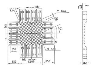
Fig.6 Shape and dimensions of typical specimen
