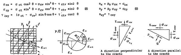
Fig.4 Average strains condition for RC plate element
