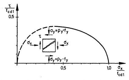
Fig. 4 Fracture criterion for a concrete element in concrete failure
