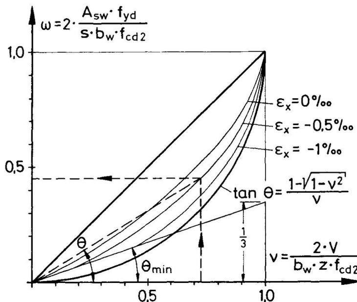
Fig. 2 Required vertical shear reinforcement in the web
