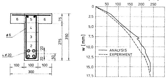
Fig.1 Cross-section, crack pattern (test and analysis) and load deflection curve of a T-beam
