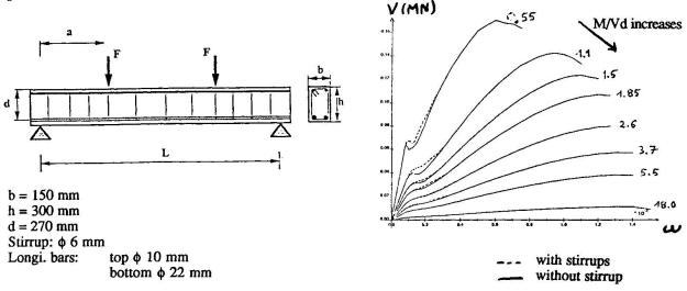
Fig.8 Beam subjected to shear
