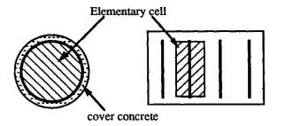
Fig.3 Hoop confined specimens
