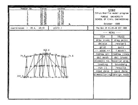
Fig. 2(a). Centerline Dimension Strut-Tie Model
