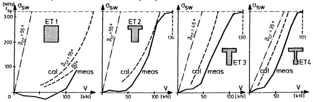
Fig.4: Development of stirrup stresses with the load for test-beams with varying web-thicknesses of Leonhardt/Walther /16/
