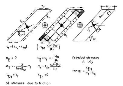
Fig.2: Forces and stresses for the concrete strut between the cracks
