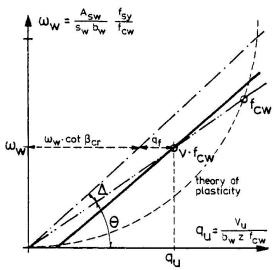
Fig.7: Interpretation of the dimensioning diagram in Fig.6 in terms of an effective concrete strength
