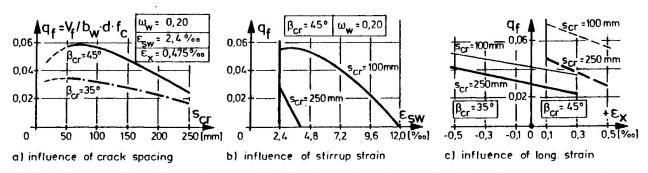
Fig.8: Influence of crack spacing, crack inclination and strains on the shear force component qf carried by friction
