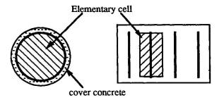
Fig.3 Hoop confined specimens
