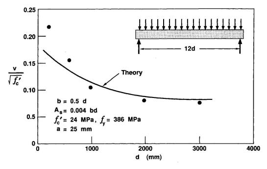
Fig. 3 Comparison of predicted and observed shear stress at failure on section distance d from the support.
