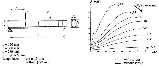
Fig.8 Beam subjected to shear
