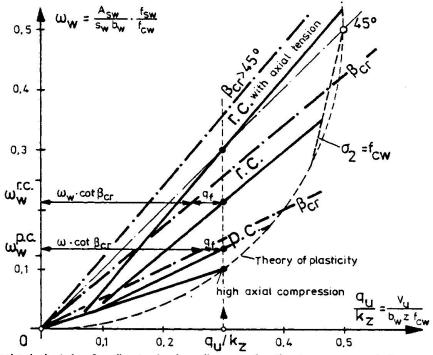
Fig.6: Principal sketch of a dimensioning diagram for the tranverse reinforcement in B-regions and influence of prestress and axial tensile and compressive forces
