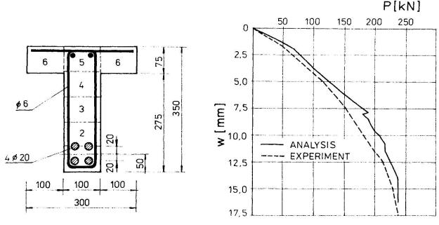
Fig.1 Cross-section, crack pattern (test and analysis) and load deflection curve of a T-beam
