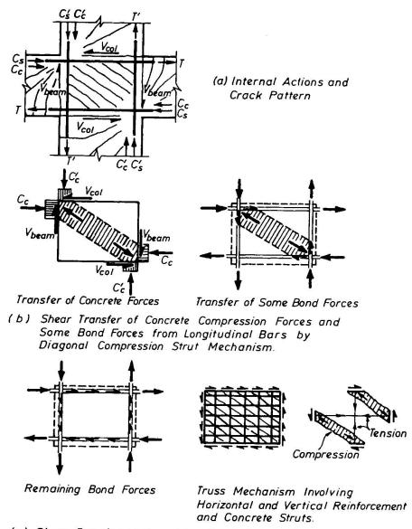
(c) Shear Transfer of Remaining Band Forces from Longitudinal Bars by Truss Mechanism.
