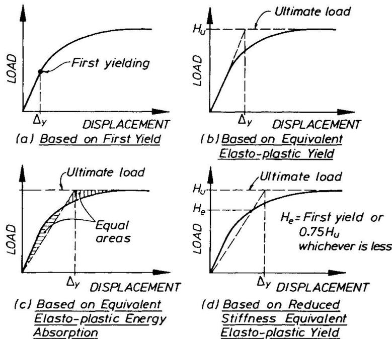
Fig.2 Alternative Definitions for Yield Displacement
