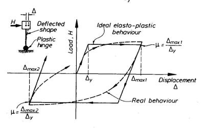
Fig.1 Displacement Ductility Factor
