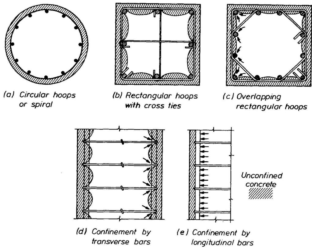
Fig.5 Confinement of Compressed Concrete by Reinforcement
