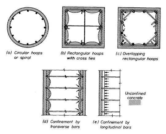
Fig.5 Confinement of Compressed Concrete by Reinforcement
