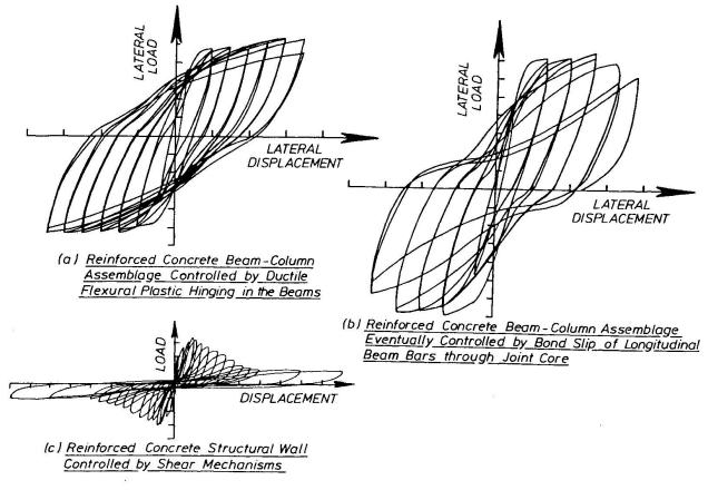
Fig. 10 - Typical Measured Hysteresis Loops for Reinforced Concrete Subassemblages
