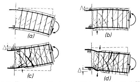
Fig.8 Significant Stages of Development of Deformations at a Plastic Hinge During Cyclic Flexure with High Shear [8]
