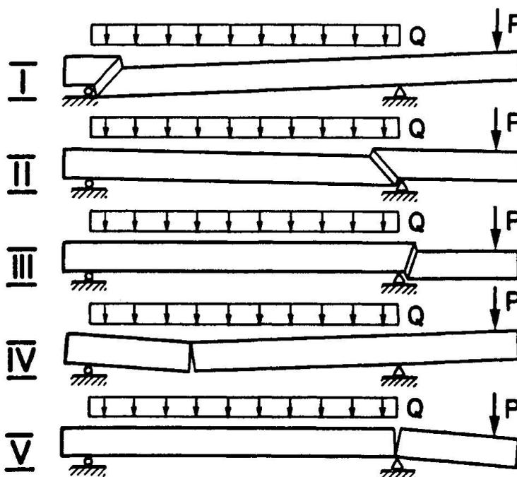
Fig. 18 Failure mechanisms for isostatic beam [6].
