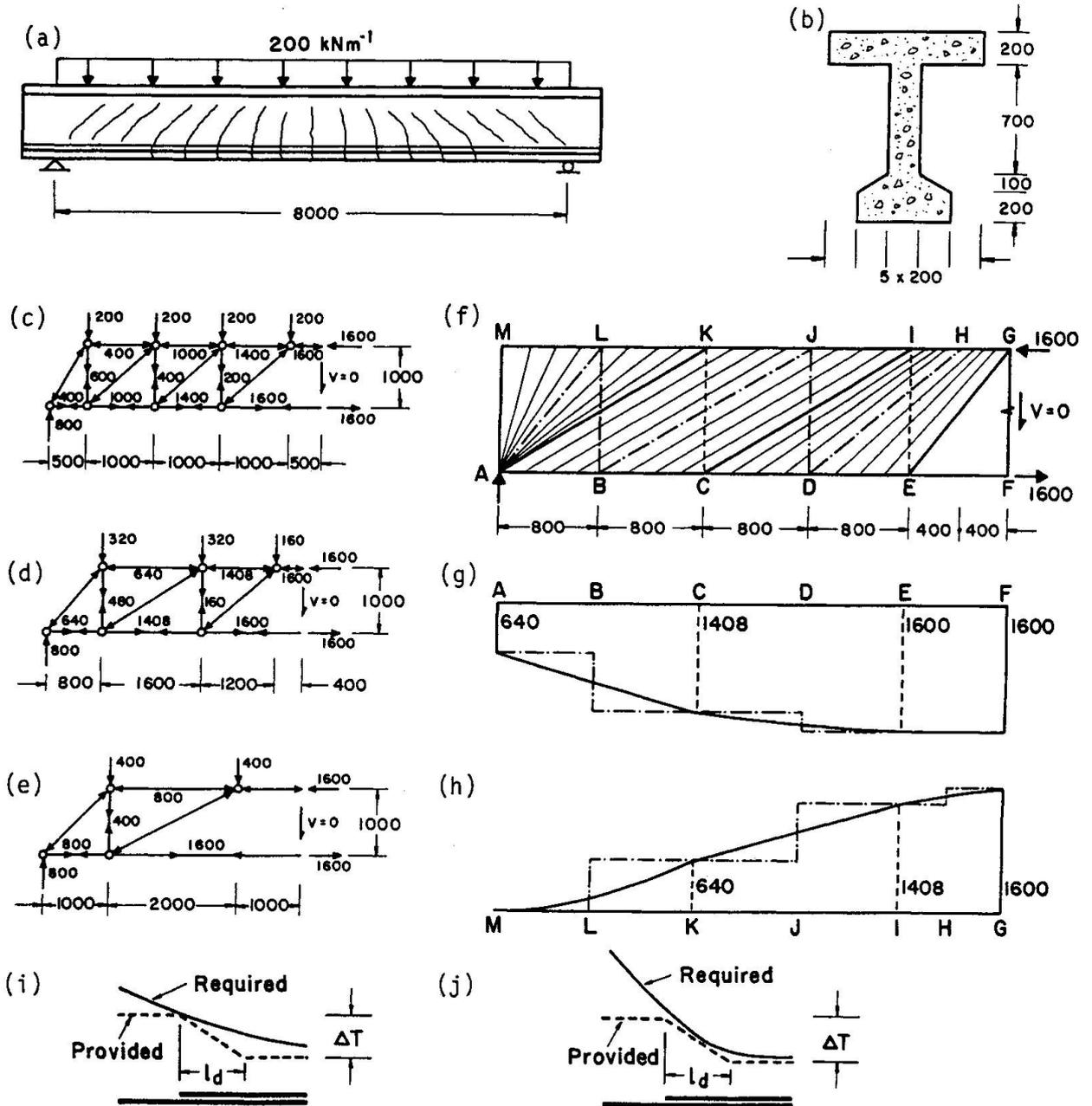
**Fig. 1** Uniformly loaded I-beam: (a) Loading and crack pattern; (b) Cross-section; (c) through (e) Truss models; (f) Discontinuous stress field; (g) Required factored resistance of bottom chord; (h) Factored top chord force; (i) Critical condition at bar cutoff; (j) Critical condition within development length.
