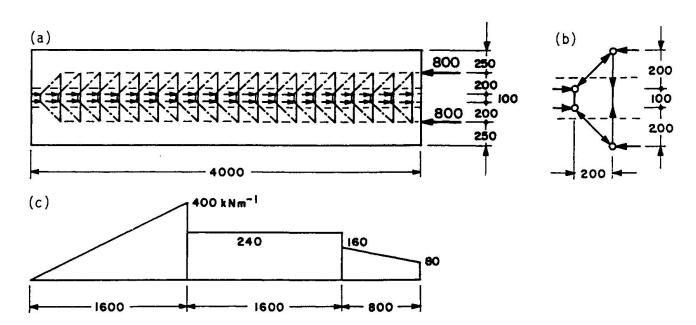
Fig. 3 Truss model for top flange: (a) Overview; (b) Detail; (c) Shear flow between web and either side of flange.
