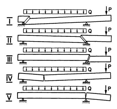
Fig. 18 Failure mechanisms for isostatic beam [6].
