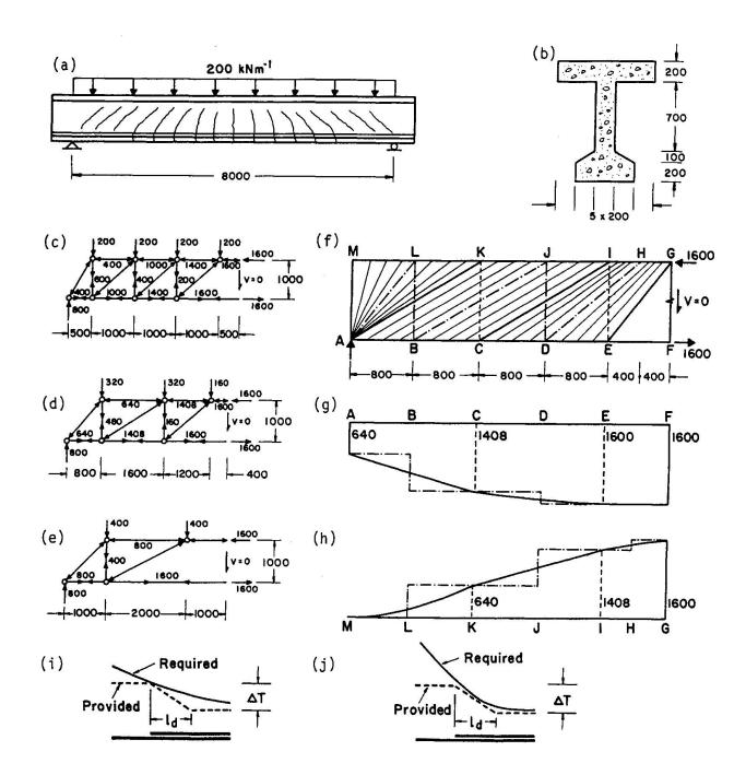
Fig. 1 Uniformly loaded I-beam: (a) Loading and crack pattern;
