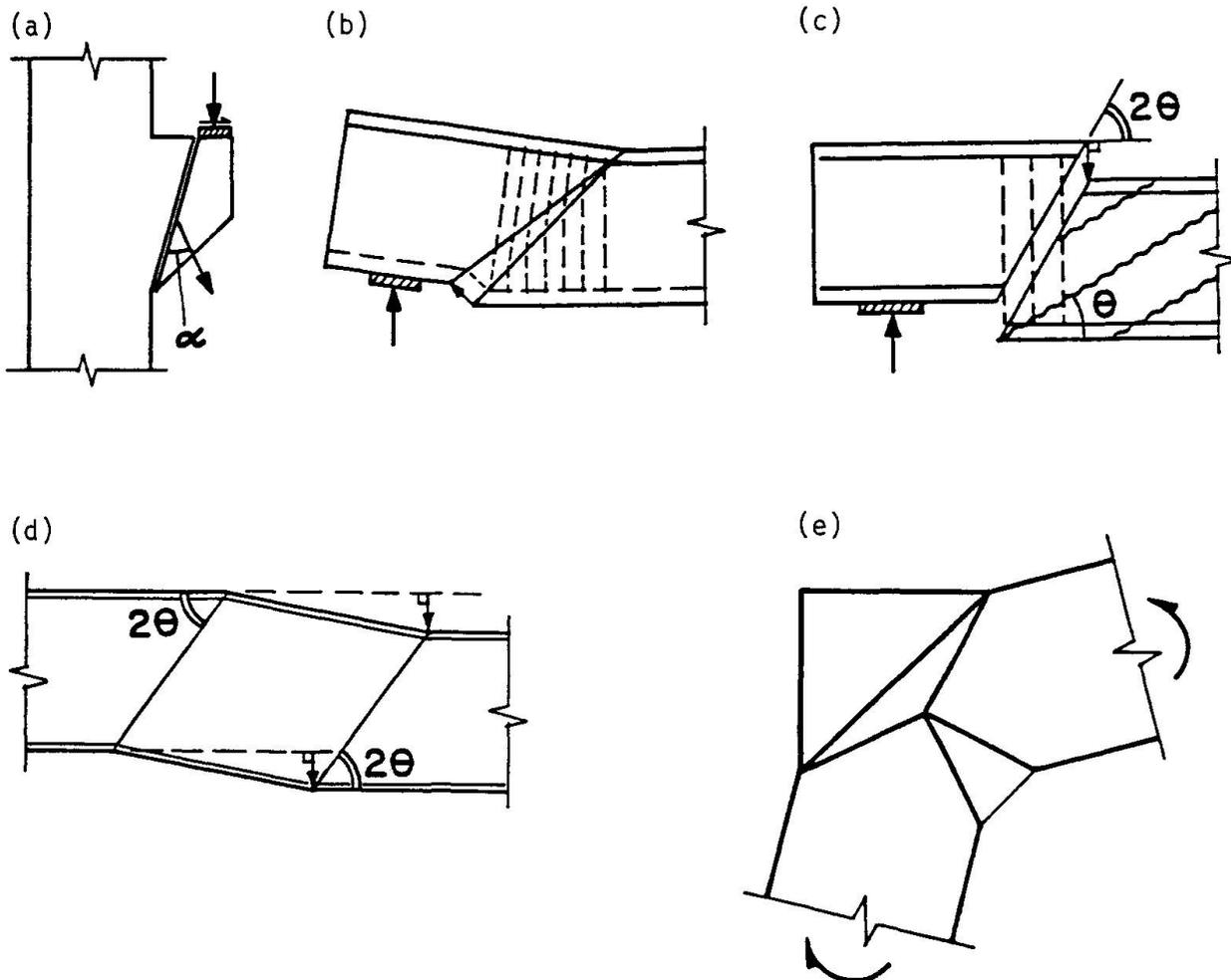
**Fig. 17** Failure mechanisms: (a) Discontinuity surface in corbel; (b) Collapse crack in beam; (c) Web crushing mechanism; (d) Web crushing and stirrup yielding in zone of homogeneous deformation; (e) Collapse crack mechanism for knee joint subjected to opening moment [41].
