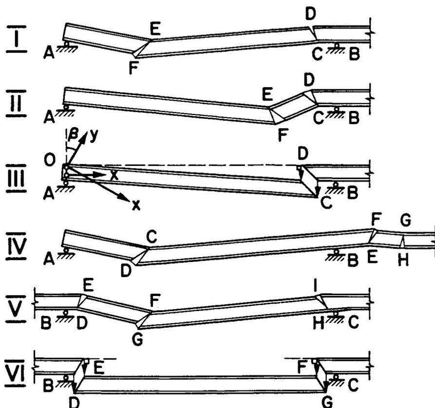
Fig. 19 Failure mechanisms for continuous girders [20].
