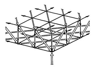
Fig. 14 Truss model for slab corner.
