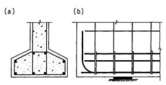
Fig. 2 Detailing of bottom chord reinforcement: (a) Cross-section; (b) Elevation at support.
