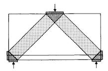
Fig. 2. Strut-and-Tie Models
