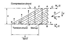
Fig. 4. Plastic Truss Model
