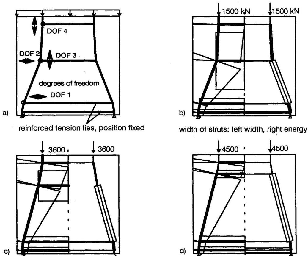
Fig. 7: Adaptation of model under increasing load
