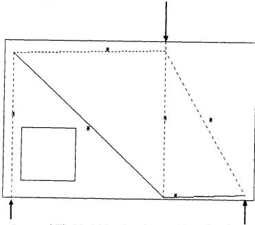
Fig.2 Strut-and-Tie Model for deep beam with perforation
