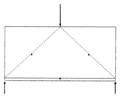
Fig.1 Strut-and-Tie Model for a deep beam
