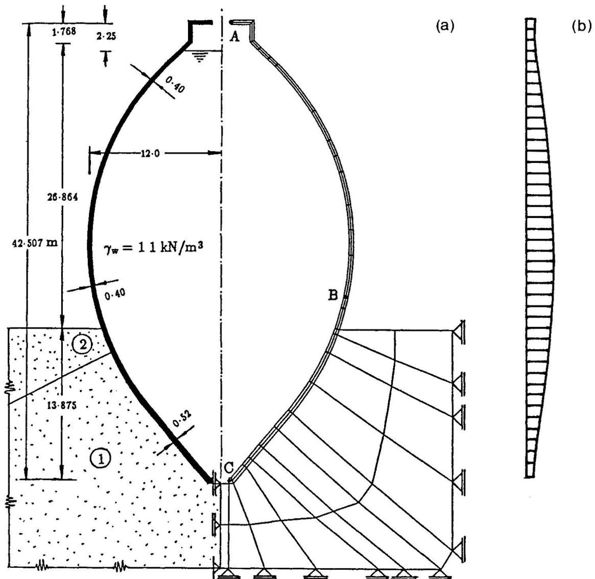
Fig.1 Prestressed concrete septic containment showing problem details and finite element idealisations: (a) axisymmetric mesh, and (b) shell element mesh.
