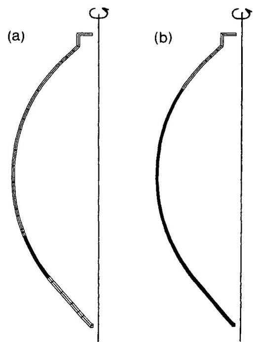
**Fig.5** Tensile cracking zones using: (a) Shell formulation, (b) Axisymmetric formulation.
