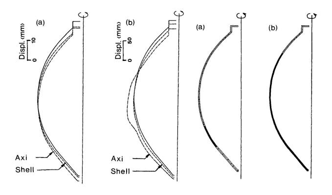
Fig.4 Deformed shapes due to: (a) Self-weight and prestressing, and (b) servis load.
