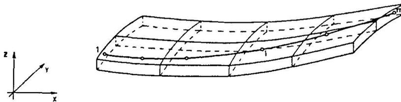
**Fig.3** Geometry of the prestressing tendon (Shell elements).
