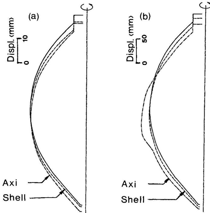
**Fig.4** Deformed shapes due to: (a) Self-weight and prestressing, and (b) servis load.
