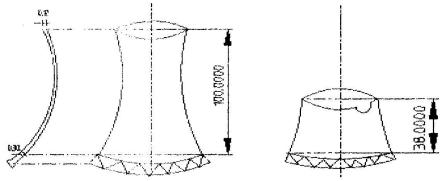
Fig.1 Cooling tower before and after collapse.
