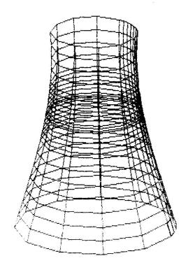
Fig. 2 a,b. Finite Element model of the discussed cooling tower.
