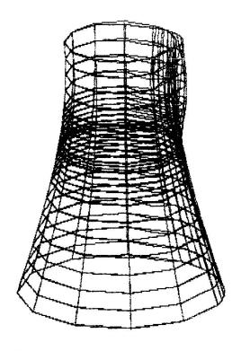
a.Displacements of the shell under the b. Zoom of the deformed wind load. Length of the slit 40 m
