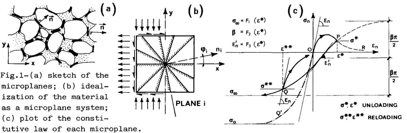
Fig.1-(a) sketch of the microplanes; (b) idealization of the material as a microplane system; (c) plot of the constitutive law of each microplane.
