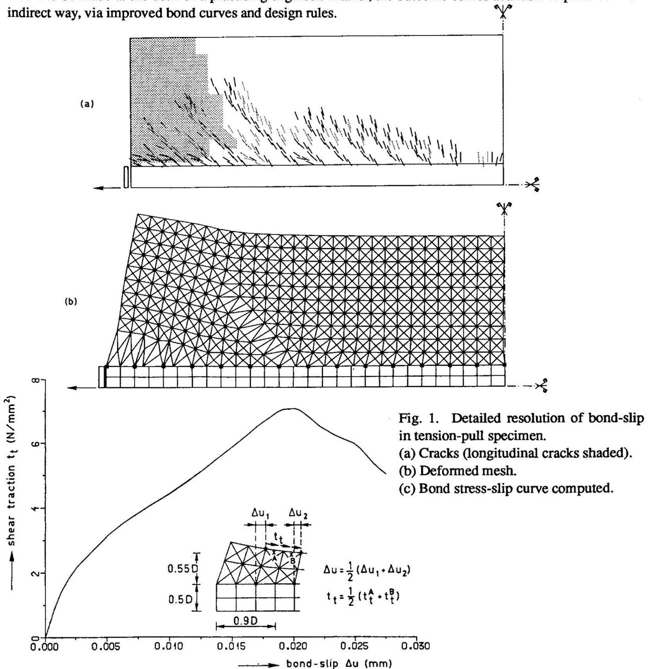
Fig. 1. Detailed resolution of bond-slip in tension-pull specimen.
