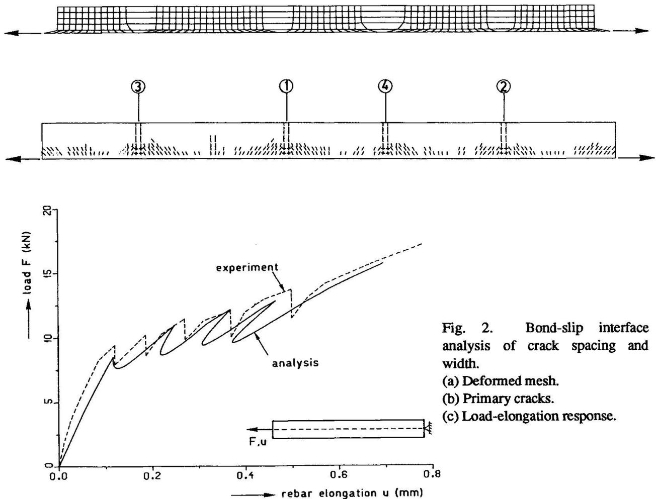
Fig. 2. Bond-slip interface analysis of crack spacing and width.
