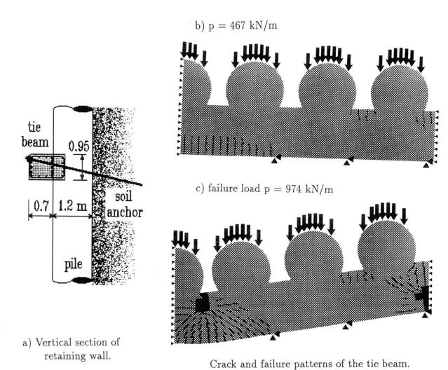
Fig.9 Simulation of the failure of tie beam supported by elastic anchors.
