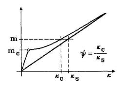
Fig.2 Moment-curvature diagram. Meanig of tension stiffening coefficient  $\psi$ .
