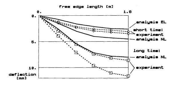
Fig.5 Comparison of analytical and experimental deflections of the free edge for Hajek's slab [3].
