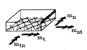
Fig.1 Moments on the cracked plate element.
