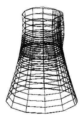
a.Displacements of the shell under the b. Zoom of the deformed wind load. Length of the slit 40 m
