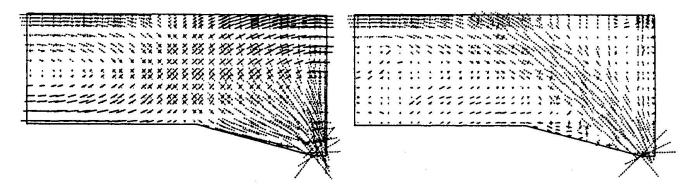
Fig. 5. Transition from linear-elastic behavior to 'strut-and-tie' system in tunnel roof.
