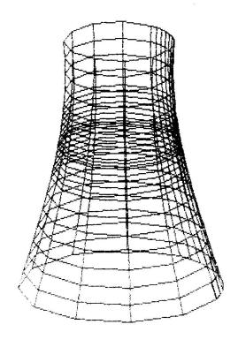
Fig. 2 a,b. Finite Element model of the discussed cooling tower.
