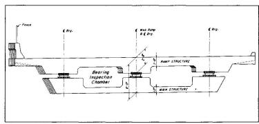
Figure 8. Cross-section through bearing inspection chamber
