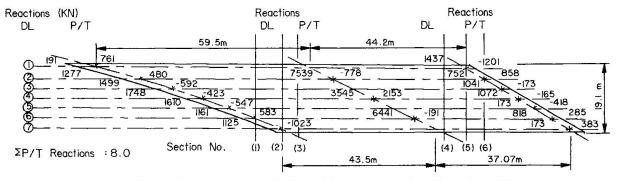
Fig. 8 Sectional Framing Plan With Support Reactions for Euclid/Park Ave. Bridge
