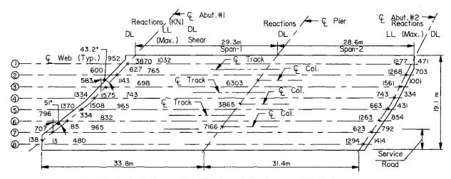
Fig. 3 Sectional Framing Plan With Support Reactions - SPRR Bridge
