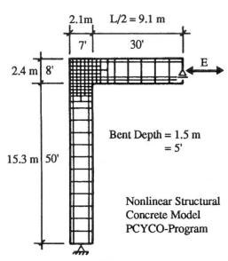
Fig. 2 Analytical bent model
