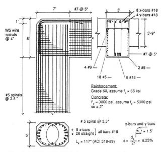
Fig. 3 I-980, #38, Reinforcement details
