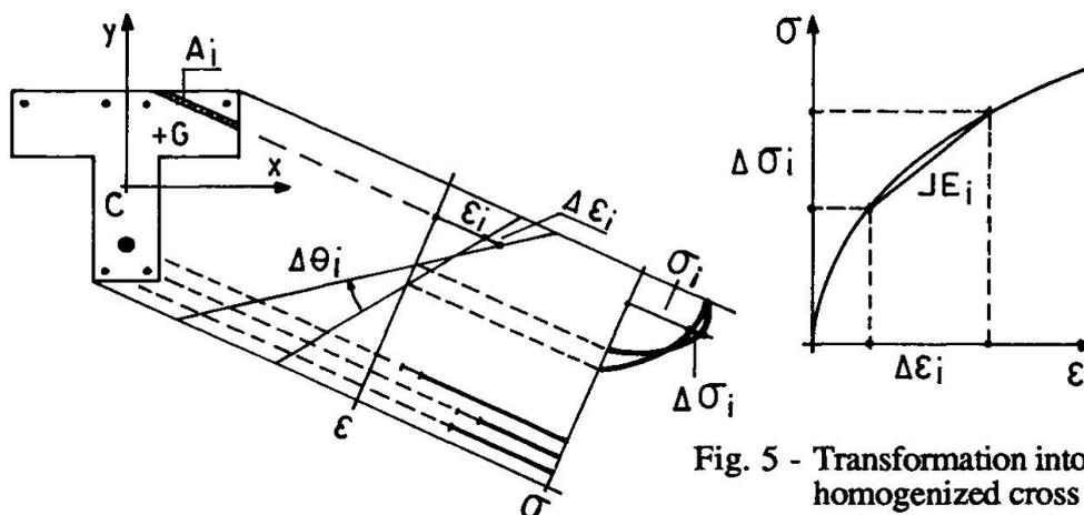
Fig. 5 - Transformation into elastic homogenized cross section
