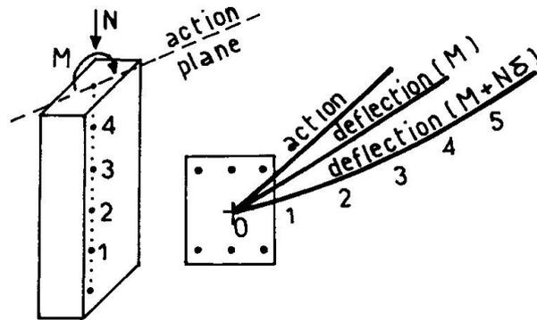
Fig. 8 - Non-plane deflection in biaxial bending
