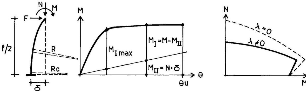
Fig. 6 - Model Column and Reduced Interaction Diagram (R.I.D.)
