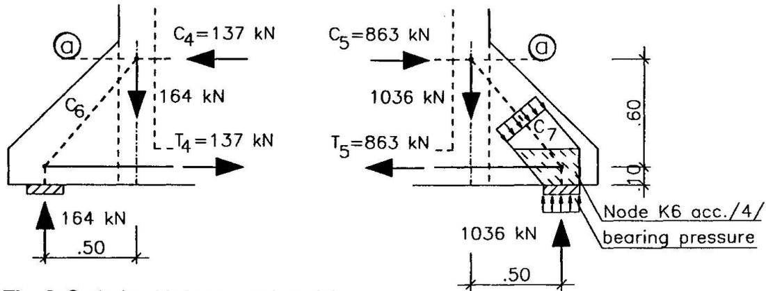
**Fig. 3: Corbels with forces and models**
