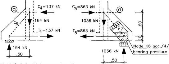
Fig. 3: Corbels with forces and models
