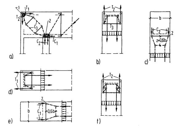
Fig. 2: Strut-and-tie models for the structure without internal diaphragm wall. a) Web; b) tensile wall; c) compression wall; d) top flange; e) bottom flange. f) Refined model for the lap problem characterized in Figs. b and d
