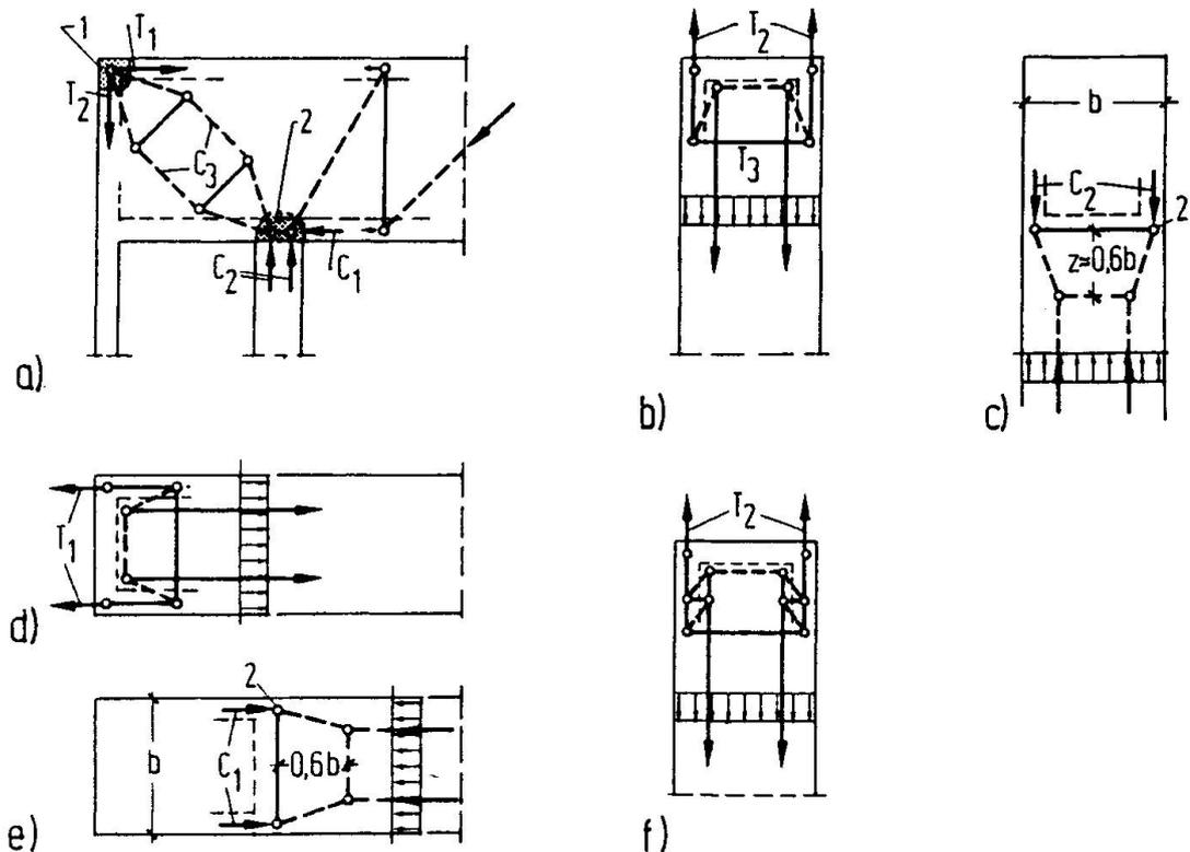
Fig. 2: Strut-and-tie models for the structure without internal diaphragm wall. a) Web; b) tensile wall; c) compression wall; d) top flange; e) bottom flange. f) Refined model for the lap problem characterized in Figs. b and d
