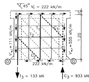
Tie forces per unit length in the diaphragm (for a  $45^{\circ}$  inclination of the compression field):  $T'_1 = T'_2 = 222 \text{ kN/m}$
