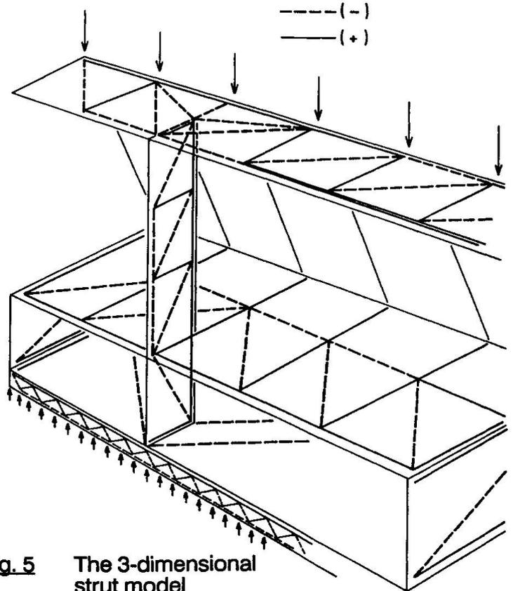
Fig. 5 The 3-dimensional strut model
