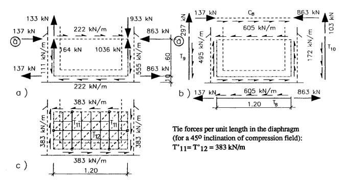
Fig. 4: Lower part of the diaphragm
