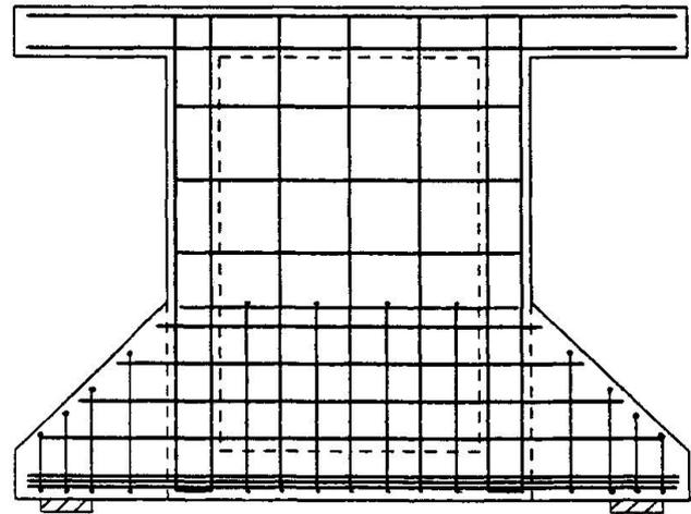
Fig. 6: Principal reinforcement layout
