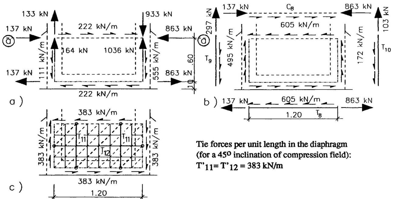
**Fig. 4: Lower part of the diaphragm**
