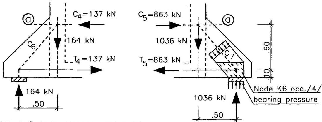
**Fig. 3: Corbels with forces and models**
