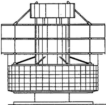
**Fig. 6** Project: suspension building of the Bayerische Rückversicherung
