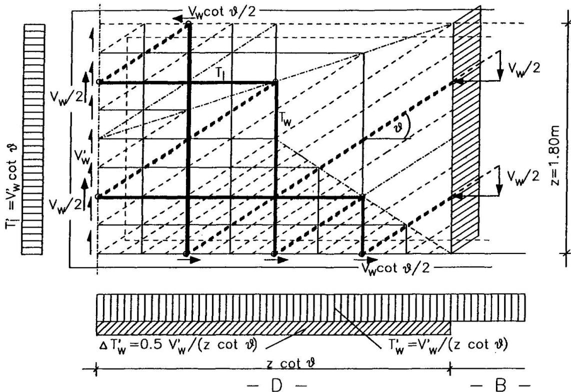
Fig. 7: Strut-and-tie-model for the webs acc. to /5/
