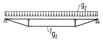
Fig. 2 Internally statically indeterminate structure loaded with g<sub>2</sub>
