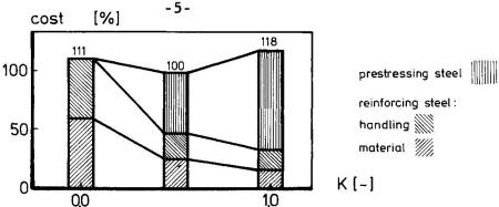
Fig. 5 Calculated distribution of reinforcement cost for three levels of prestress (100% = dfl. 5200, - = US\$ 2500, - dated Oct. 1988).
