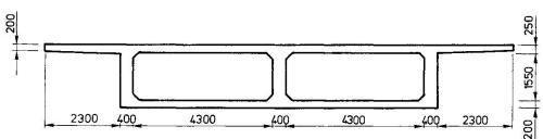
Fig. 6 Cross-section of the box-girder bridge.
