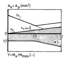
Fig. 2 Reinforcement ratio and  $\gamma$  as a function of the degree of prestressing.
