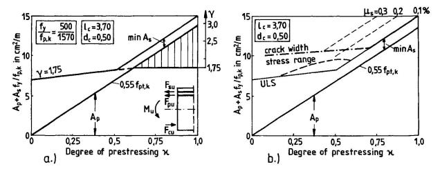
Fig.4: Proportional amount of reinforcement in a posttensioned cross-section a.) from the check of the load capacity (ULS)
