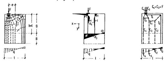
Fig. 3: A typical D-region: (a) elastic stress trajectories; (b) elastic stresses; (c) strut-and-tie-models.
