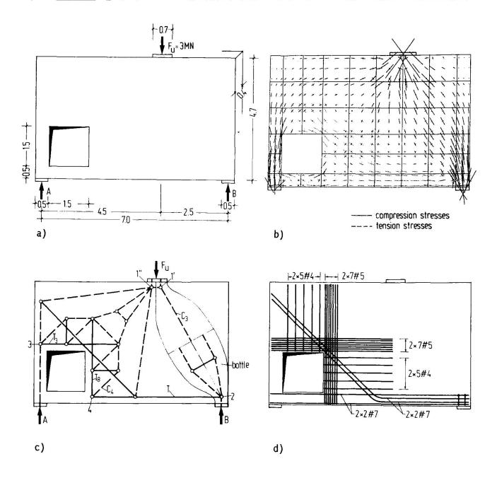
Fig. 6: Deep beam with a large hole. (a) dimensions /m/ and load; (b) elastic stresses; (c) complete strut-and-tie-model; (d) reinforcement.
