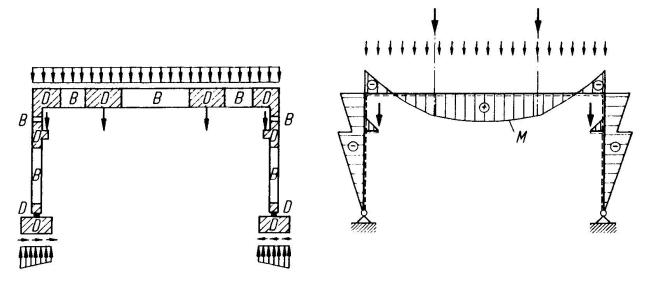
Fig. 1: A frame structure containing a substantial part of B-regions, its statical system and its bending moments.
