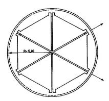
Top slab at erection state with eccentric loading Fig. 7
