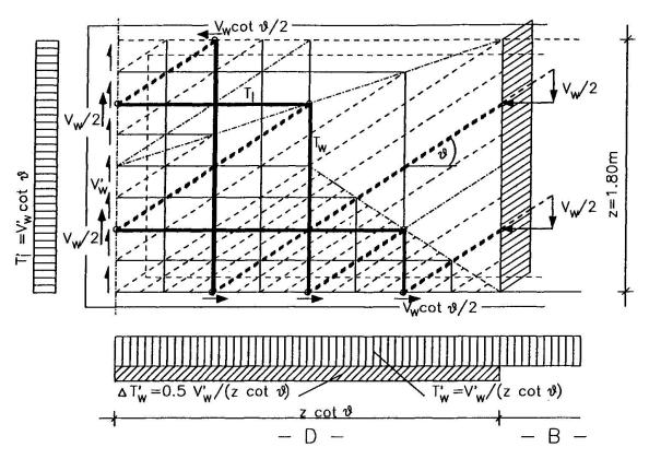
Fig. 7: Strut-and-tie-model for the webs acc. to /5/
