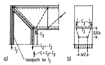
Fig. 5: a) Diagonal diaphragm following the load path for T<sub>2</sub> of the strut-and-tie model. b) Model for the compression wall.
