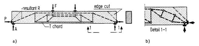
Fig. 8: (a) Strut-and-tie-model of partially prestressed beam with rectangular cross section; (b) detailed strut-and-tie-model of the beam area, where the resultant is within the beam section.
