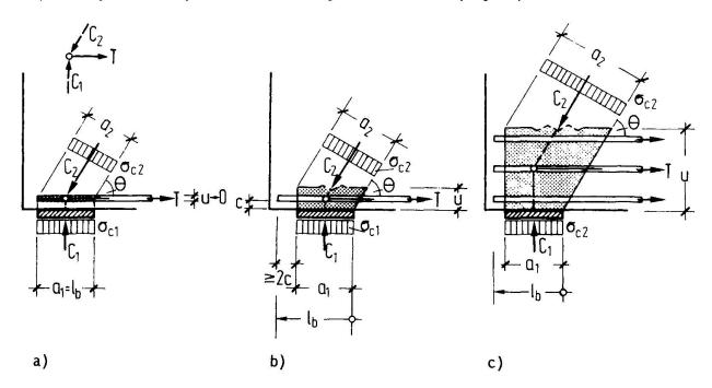
Fig. 7: Typical node for the anchorage of reinforcement; (a) one layer; (b) one layer with additional length behind the node; (c) three layers with additional length behind the node.
