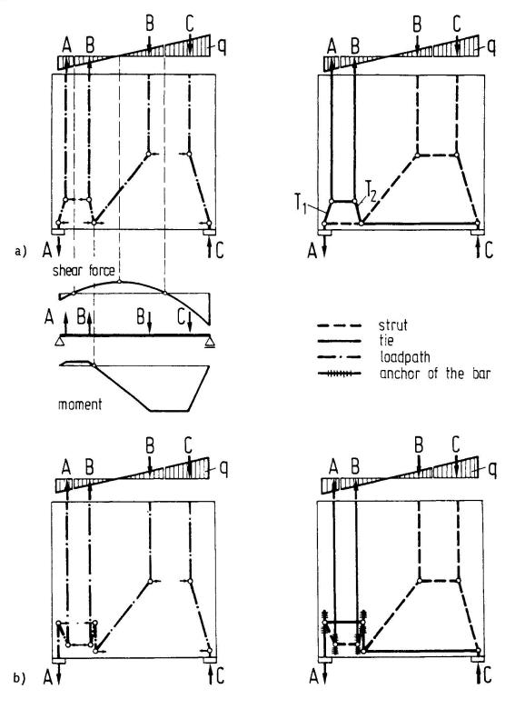
Fig. 5: Application of the load path method for finding the appropriate strut-and-tie-model. Two models for the same case: (a) requiring oblique reinforcement; (b) for othogonal reinforcement.
