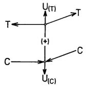
Fig. 13 Forces U due to change of direction
