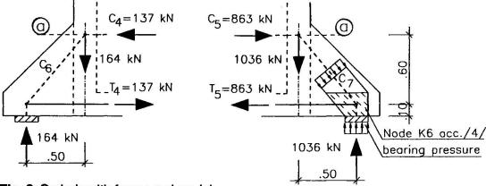
Fig. 3: Corbels with forces and models
