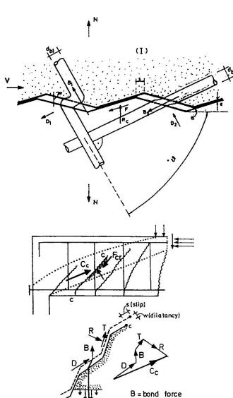
Fig. 3: Topology (a) and forcedisplacement output (b) of an interface model
